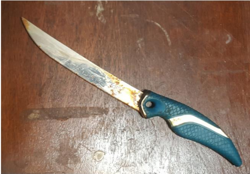
No mercy was shown to this Cuda knife, and as you can see, a year later there's some surface rust at the tip, along the blade, and near the handle.
